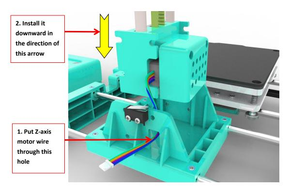
2. After insert the XZ Axis, Fixed with 2 screws.
