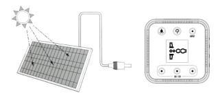
▲ The solar input can handle up to 18V5A(90W Max.) per hour,recharged with 100w panel in 4-5 hours to full under straight full sun (3 hours, under STC, AM1.5, 1000W/m² 25℃,recharging time varies from different location, temperature ,weather,etc.).
