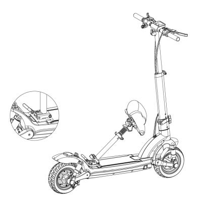
4. Lift up the seat until it locks in place. Loose the bolt to adjust the height of the seat. Once the required height is reached, tighten the bolt. Verify that the seat is locked in place by pulling upward on the seat. If the seat is properly locked, the seat will not move up or down.
