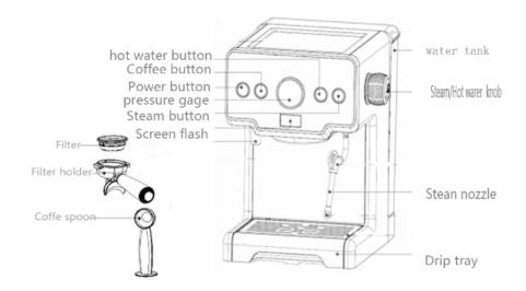
Warning: The machine must use a grinding Coffee powder and is composed of a central structure for obtaining espresso and steam/hot water.
