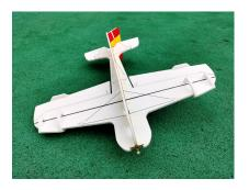
9. Glue on the 4 carbon rods on the front of the fuselage. Before the glue solidifies, make sure that the horizontal and vertical parts of the fuselage are vertical.
