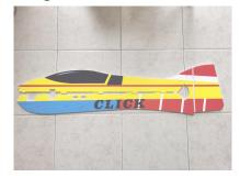
6. Stick the wing and fuselage together, and pay attention to the fact that the wing and fuselage must be vertical.
