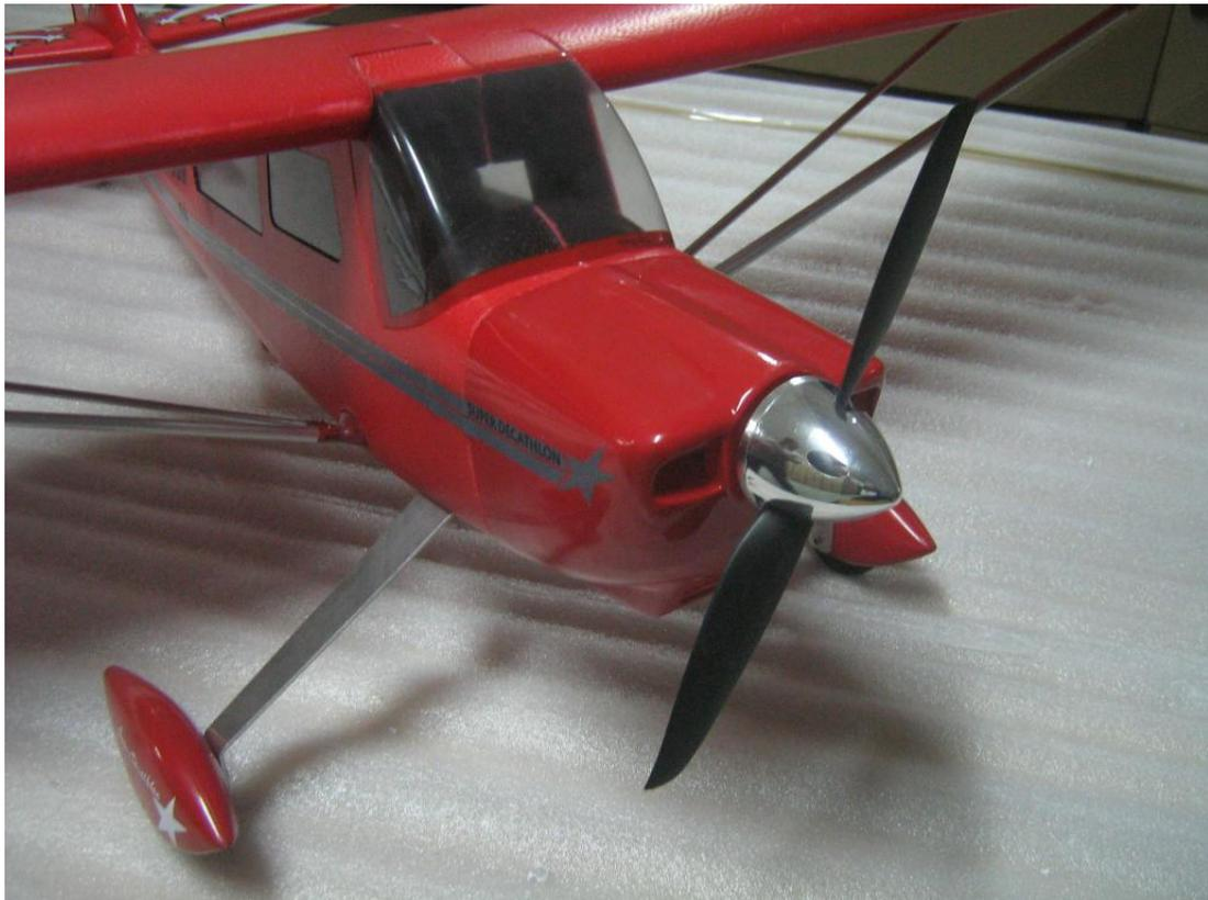
4, Assemble the landing gear (floats struts) under the fuselage with M4\*25 screw.
