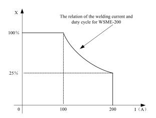
output an instruction to cut output welding current, and brighten the over-heat pilot lamp on the front panel. At this time, the machine should be relaxed for 15 minutes to cool the fan. When operating the machine again, the welding output current or the duty cycle should be reduced.
