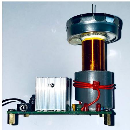
Figure 3: The finished Tesla coil/plasma speaker
