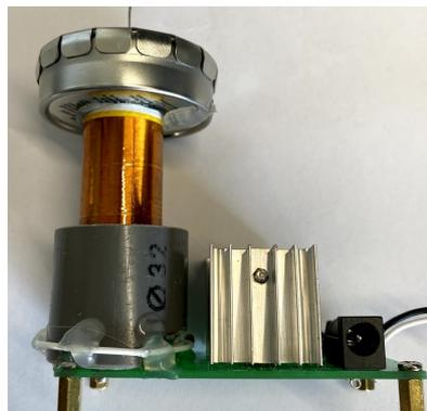
Figure 5: Lowered L1 winding reduces coupling, increases sparklength
