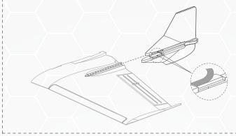
2. Secure the wings with the provided double-side tape. Remember to first run the main spar through the fuselage.
