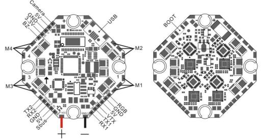
Babyhawk II HD's main electronic board is shown above. This board contains a F4 flight controller with all 4 esc's.
