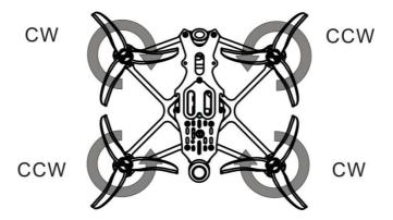
**Caution:** Failure to mount the propellers in the correct orientation will cause Babyhawk II HD to not fly correctly and with no control. Please double check for the correct orientation.
