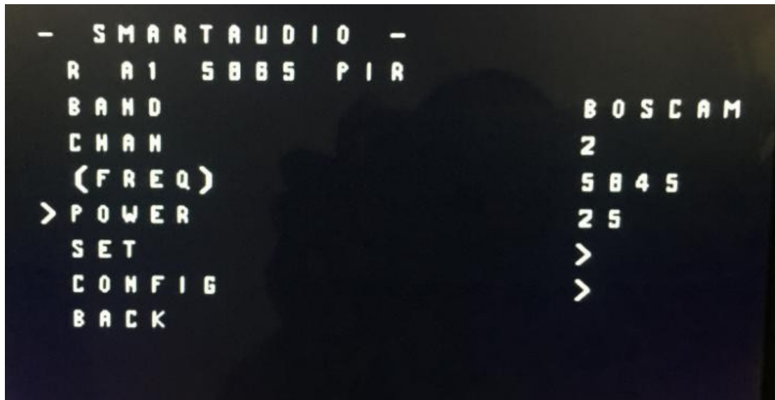
Figure 7 Transmission Power Selection
