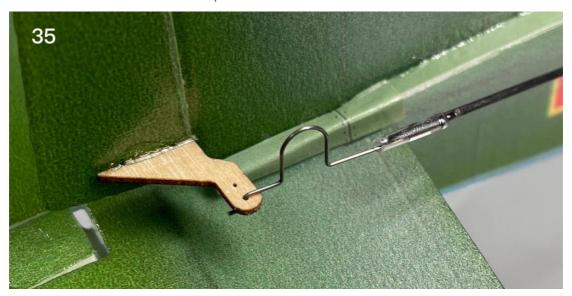
36. Install the aileron control horn.
