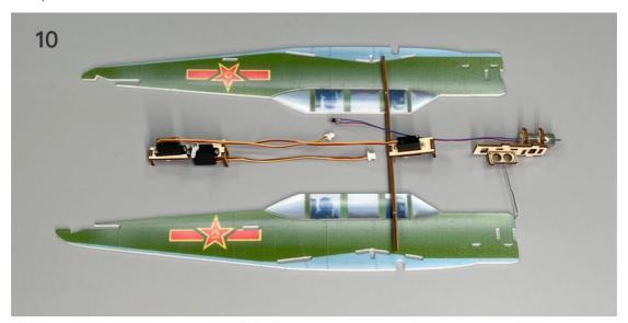
11. Install the fuselage internals according to the marked position inside the fuselage
