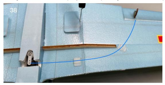
39. Use 502 glue to fix the conduit on the base. Note that 502 glue is not accessible to foam parts.
