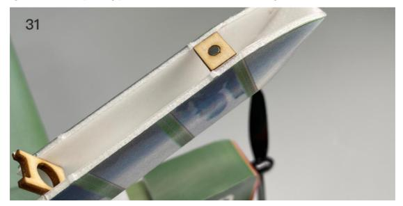
32. Install control horns on the rudder and elevator.
