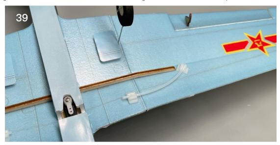
40. Aileron wire drive system. Bend the steel wire as shown to decrease resistance.
