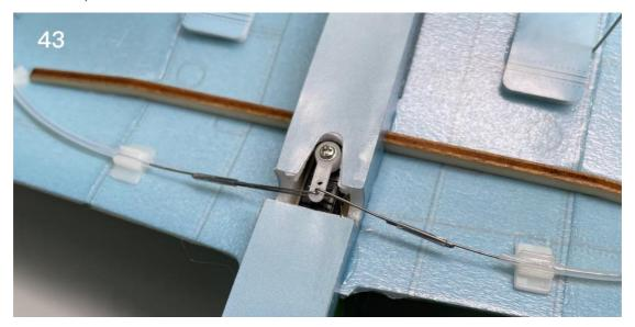
44. Connect the aileron servo to a powered receiver to make sure the servo arm is on its central position. Connect the steel wire and clips with heat-shrinkable tube and fix with glue. (Note: Using fire may damage foam material. Please use electric soldering iron.)
