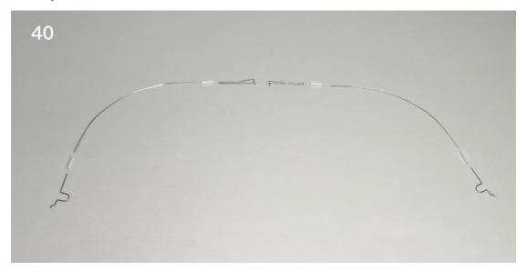
41. Connect the steel wire and a servo clip with heat-shrinkable tube and fix them with 502 glue.
