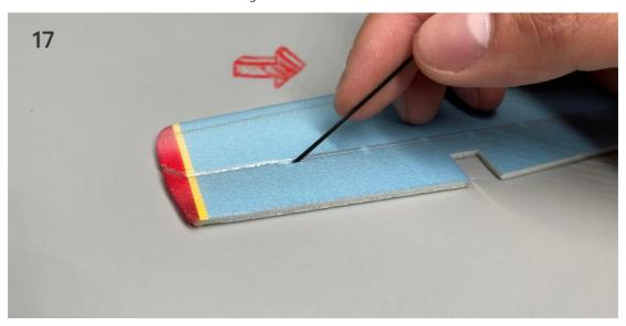
18. Install the tail. Make sure the horizontal tail is parallel to the fuselage and the vertical tail is vertical to the fuselage.
