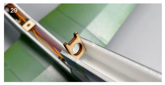
30. Fix the magnet on the fuselage with the magnet holder.
