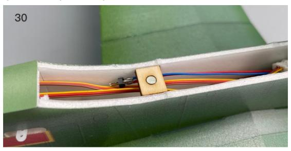
31. Fix the magnet in the corresponding position of the hatch cover with the magnet holder.
