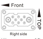
1 Aileron 2 Throttle 3 Flap 4 5V+ 5 GND 6 AUX 7 Throttle GND 8 AUX 9 Battery + 10 Battery -
