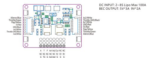
The left and right side Aileron, Throttle, Flaps signal are parelled.
