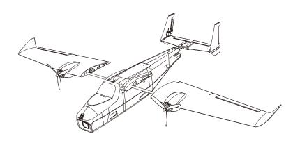
Detachable wing and tail Also with power and signal connector, no more mess up wires, quick deploy.
