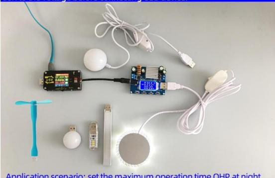
Application scenario: set the maximum operation time OHP at night, and turn off the output automatically when the time is up.
