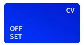
CV: default regulating voltage, long press set button for 1 second to adjust constant
