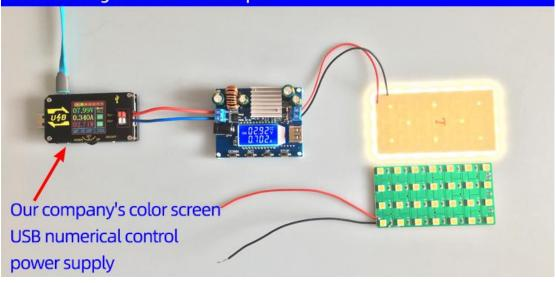
It is used as a common voltage regulator with over-voltage / over-current / over power / over temperature / under voltage protection.
