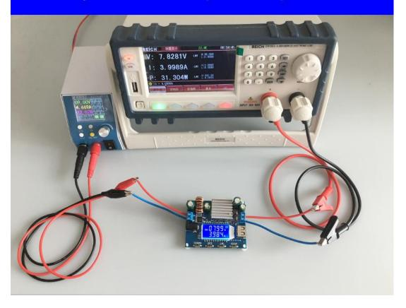
Product with USB female output, convenient for USB device access The voltage of USB port is the same as that of terminal. Please pay attention to the voltage before connecting USB device.
