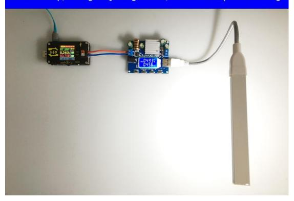
USB Fan, through adjusting the voltage or current, realize the stepless speed regulation of the fan!
