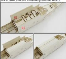
3.Take out C2, D3, E4 from the board, install the bottom cover over the fuselage frame, use glue to stick the junction, assemble A20 at the same time, put the magnet (G8) into the inside of preformed hole.
