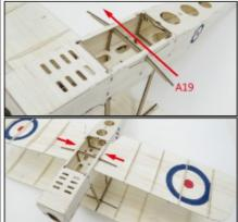
6.Take out A12 from the board, install the top wing and under wing as below pictures, use glue to stick the junction, and install emulational parts.
