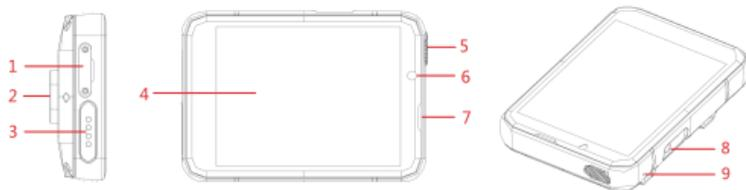
1.Nano SIM card slot; 2.Heart rate sensor; 3.Magnetic charging; 4.Display; 5. Power key; 6.Front camera;
