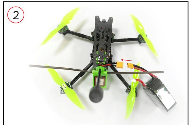
2. Connect the battery to the NOVICE-IV Drone, and make sure to fixed the battery properly with the Lipo strap.
