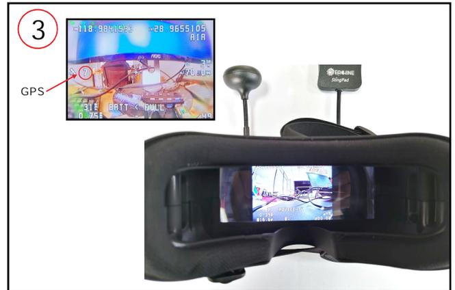
3. Turn on the EV800DM Goggles, check the video and the status of the oSD info , Make sure GPS must search for more than 6 satellites to lock the home position .
