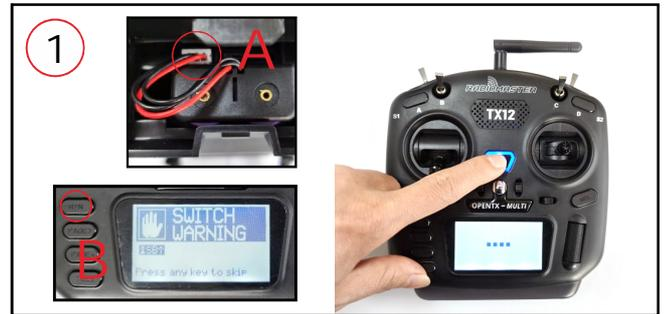
1. Install the battery to the radio(shows on picture A), and turn on the "power switch", Press any key to skip if any alarm(show on the Picture B) appear on the screen
