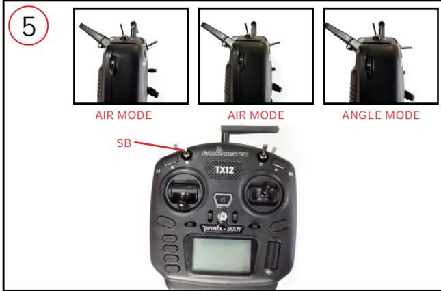
5. Toggle the SB switch to change the flight mode (Default is Air mode). We highly recommend to use Angle mode for the beginners. The motors will auto-spin when armed if the flight mode is AIR MODE.
