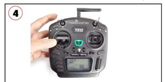
4.Keep the throttle stick lowest point and then toggle the SE Switch to Arm the NOVICE-IV drone, you will find "ARMED" notice on the screen of the goggles. Happy flight and keep it safe.
