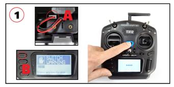
1.Install the battery to the radio(shows on picture A), and turn on the "power switch", Press any key to skip if any alarm(show on the Picture B) appear on the screen
