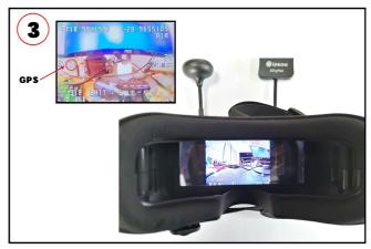
3.Turn on the EV800DM Goggles, check the video and the status of the oSD info , Make sure GPS must search for more than 6 satellites to lock the home position .
