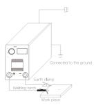
3. Correctly connect the arc torch or holder according to the sketch. Make sure the cable, holder and fastening plug have been connected with the ground. Put the fastening plug into the fastening socket at the "-" terminal and fasten it clockwise
