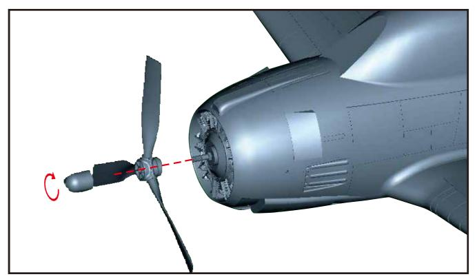
Note: It is recommended that you balance the prop and spinner before installing for optimum performance and efficiency.
