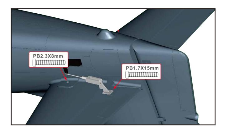
4. Locate the bag marked "Rudder" Install the control horns on the vertical tail. Connecting the pre installed control rods to the outer hold of the control horn.
