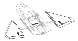
Mount the main wings with the provided thumbscrews. Don't forget to place the main spar first.
