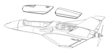
Once you placed all your FPV gear, be sure both hatches fit flushed against the fuse.
