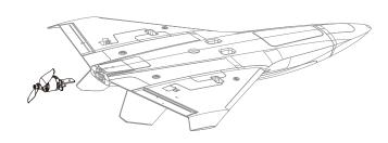
You will fix the motor seat with the 2 provided screws. Be sure is aligned and firmly tighten.
