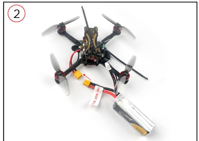
2. Connect the battery to the NOVICE-III Drone, and make sure to fixed the battery properly with the Lipo strap.
