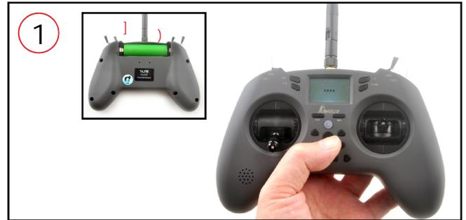
1. Install the battery to the radio (Make sure not to connect the wrong polarity of the battery), and turn on the "power switch", short press "RTN" button if any alarm appear on the screen to continue.
