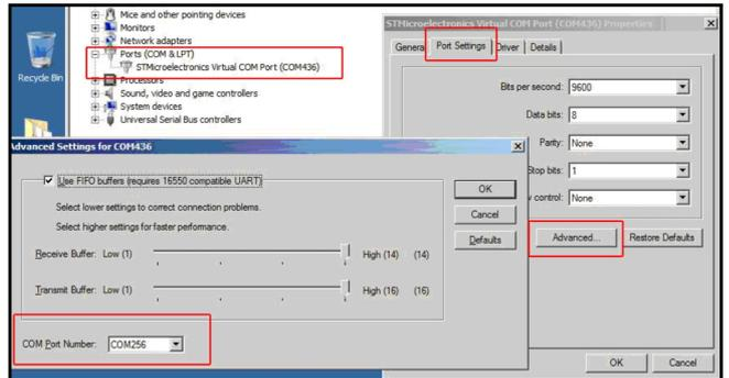
4. Open the BLHELISUITE, Select SILABS BLHeli Bootloader (Cleanflight) from the third tab on the top side. Then Select the right Serial com port and Click connect. You can also Flash the new release BLHeli\_s firmware via the BLHELISUITE, the firmware Target is "F-H-40"
