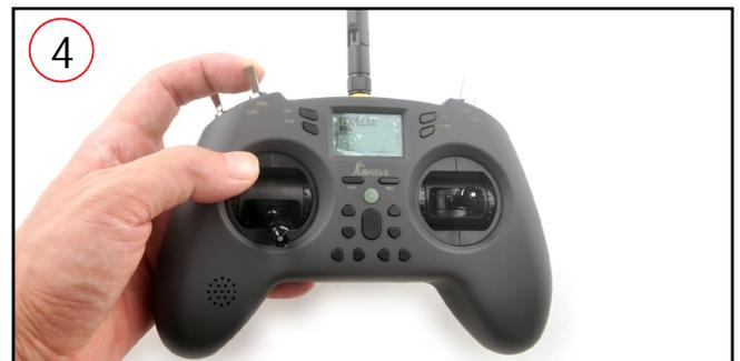
4. Keep the throttle stick lowest point and then toggle the SWA Switch to Arm the NOVICE-III drone, you will find "ARMED" notice on the screen of the goggles. Happy flight and keep it safe.
