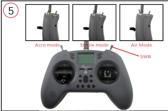
5. Toggle the SWB switch to change the flight mode (Default is Acro mode). We highly recommend to use stable mode for the beginners. The motors will auto-spin when armed if you selected the Air mode.
