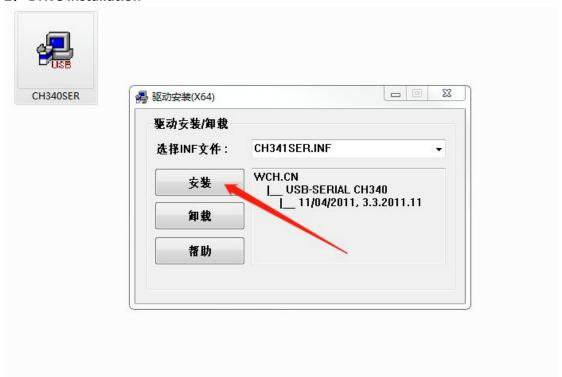
Double click the left mouse button to install the driver file. After the installation is successful, open the device manager, and the linked machine will display the control board port, indicating that the driver file has been successfully installed.
