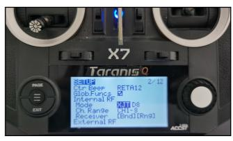
3) Check the receiver channel map and channel value is correct after bind successful.
