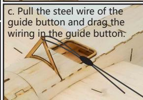
c. Pull the steel wire of the guide button and drag the wiring in the guide button.
