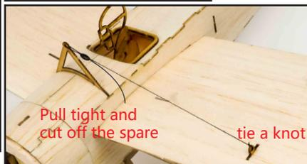
d. Pull one wiring to the hole on the wing and tie a knot, and pull the other wiring tight and keep suitable length, finally cut off the spare.
