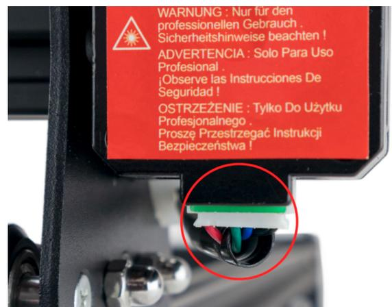
**IMPORTANT:** Use the following illustration to confirm that the XH2.54mm Connector is seated properly into the X-Axis Stepper Motor. If you notice any angle in the connector please press the connector further with your fingers until its parallel with the Stepper Motor body.
