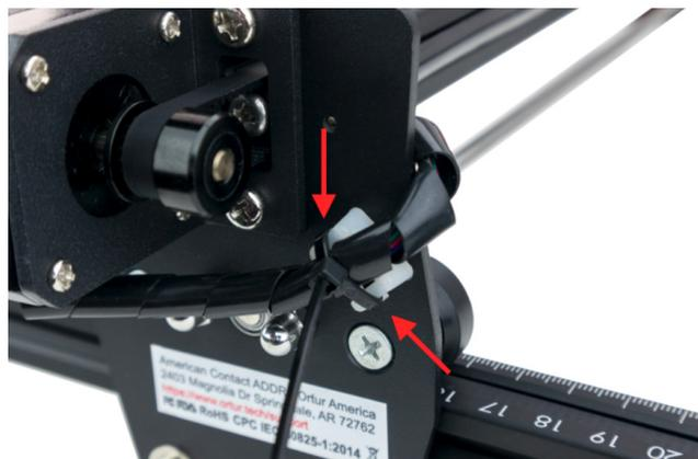
Confirm the Cable Ties are as tight as possible without using any additional tool. With your Flush Cable Cutter trim the Cable Ties so no excess is left.
