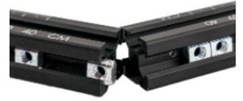
2. Slide 4x Profile Corner Brackets into the joining corners of all rails. Do note, as shown on Highlights #3 #4 #5 and #6 each corner will require a specific orientation of the Profile Corner Bracket. If sliding the Corner Brackets seems difficult, use the 2.5mm Hexagon Wrench to adjust the tightening bolt. **Do not tighten the Profile Corner Brackets at this step.**
