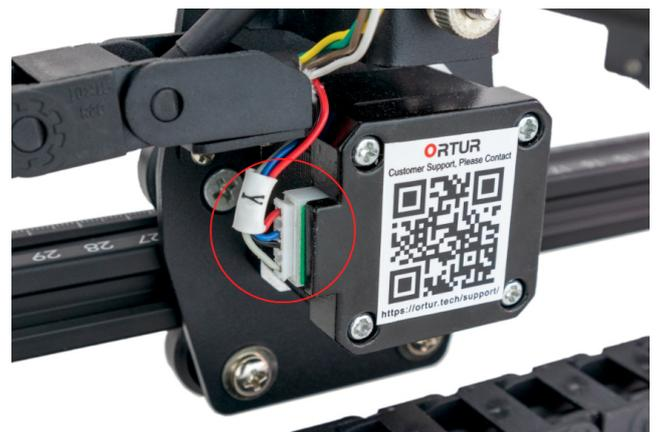
**IMPORTANT:** Use the following illustration to confirm that the XH2.54mm Connector is seated properly into the Y-Axis Stepper Motor. If you notice any
