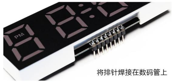
11. Check if there are any problems with the components and solder joints, and then install the digital tube
