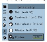
As shown in the figure, press " MENU " key to enter the main menu and select "  $\mathcal{E}$  " (emissivity) option and press "  $\blacktriangleright$  " key to enter the emissivity list.
