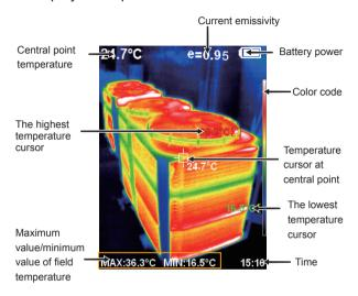
Color code: used to mark the color corresponding to the relative temperature from low to high in the field of version.
