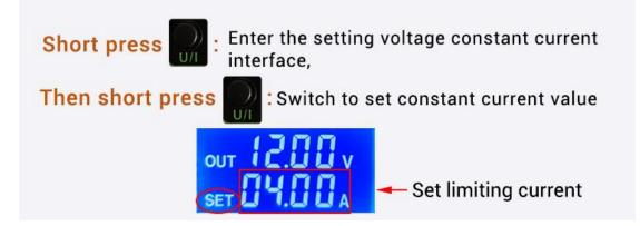
7.4. Set the default on / off state of the module when it is powered on——In the normal interface, long press the U / I key to enter the parameter setting interface. You can see the display OPEN OFF or OPEN ON. OPEN OFF represents the power on default off output, and OPEN ON represents the power on default on output. Long press rotary encoder to switch between two states. After setting, long press the U / I key to return to the normal interface.
