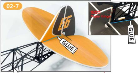
在机身尾部安装水平尾翼与垂直尾翼,并用泡沫胶粘固,粘贴时保持两个尾翼相互垂直。 Install the horizontal tail and vertical tail at the rear of the fuselage and stick with foam glue, and maintain the two tail wings perpendicular to each other when pasted.
