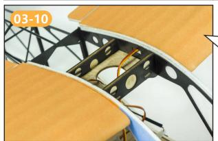
舵机线按上图放置,引导到舱身位置。 The servo line is guided to the position of the fuselage body according to the position shown in the figure
