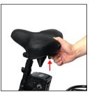
①Press the quick release button to release the seat
