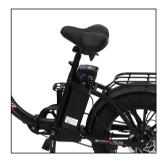
A.Recharge the battery on the E-bike directly
