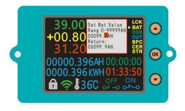
2: click the lower key to switch the parameter adjustment bit, click the upper key to change the parameter value, when the return value and the set value are the same as the data sent successfully, click the OK key to exit the parameter save, At the same time, the buzzer will send an alarm to indicate that the parameter is saved successfully.
