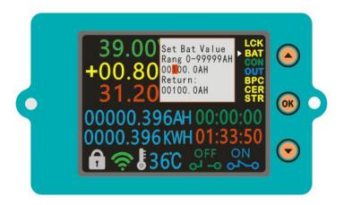
Parameter setting method 2: here according to the set communication channel value FCH as an example, how to set parameters;
