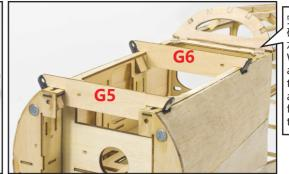
安装F12.W-A时,可用装配工具 确定角度,调整好角度后,用胶 1水粘固,最后取下装配工具。 While installing F12.W-A, use assembly tools to determine the angle, after adjusting the angle, use glue to fix it, and finally remove the assembly
