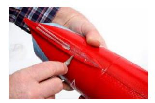
12. Epoxy the fin in position make sure to feed the left elevator pushrod tube through the fin.
