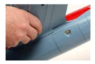
8. Make sure that the wing panel is fully inserted into the fuselage. Check both the top and bottom surfaces of the wing to be sure.
