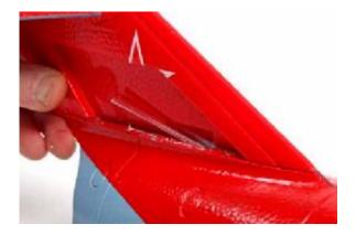
13. Slip the right elevator pushrod tube through the other fin part and glue into position.
