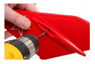
5. Apply a little epoxy to one end of the tube and insert it through the fin and into the stab. Drill the left stab in the appropriate location and slip it on the carbon tube and glue to the fin.
