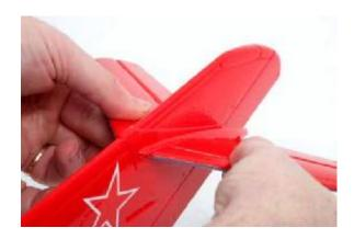
6. Check that the stabilizers are at 90 degrees to the vertical fin. Mix some 5-minute epoxy and apply an even coat to the root of one wing panel.
