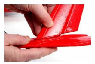
4. Check that it is at 90 degrees from the fin. When the epoxy has cured drill a 3mm hole through the vertical fin from the left side. Drill a hole inside the stab to accept the 3mm carbon tube reinforcement.
