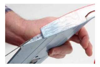
7. Insert the aileron servo wire through the hole in the fuselage and then push the wing panel into position
