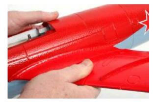
9. If there are any places where the epoxy has been forced to the surface. Take a paper towel and some Alcohol and wipe it off before the epoxy sets.
