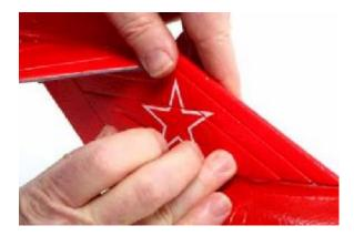
14. Insert the wire pushrods from the rear and feed them into the hatch area of the fuselage. 15. Slip both pushrods into the pushrod keeper do not tighten yet.
