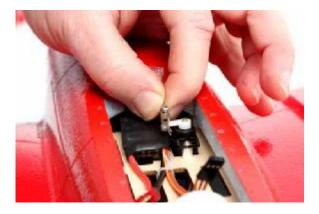
16. Insert the pushrod wire in the elevator keeper and tighten. While holding the elevator halves in neutral position tighten the keeper at the servo to pinch both wires.
