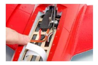
20. Install your receiver. Ailerons can be plugged in either using a Y-connector or to individual channels depending on what radio you choose.
