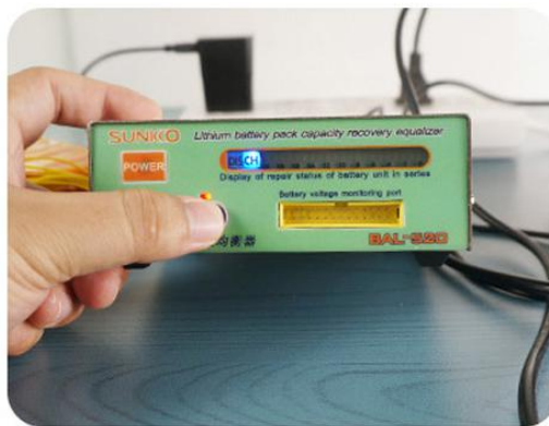
6. Press CH/DIS to switch to discharge mode (In charging mode, the CH/DIS working light is on, and the indicator light will be on when the battery is fully charged)
