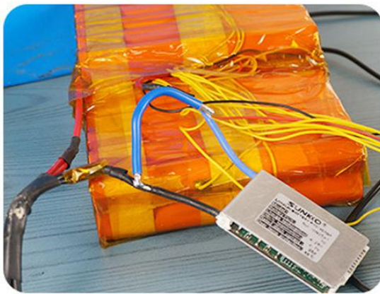
1. Short circuit the battery pack protection board (the protection board needs to be disconnected during the charging equalization process)
