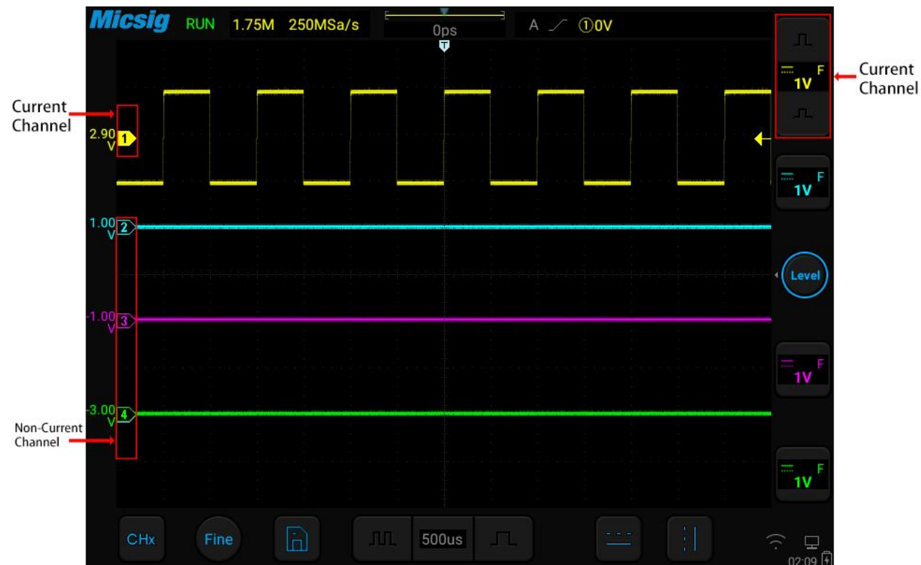
Figure 5-2 Current Channel and Non-Current Channel
