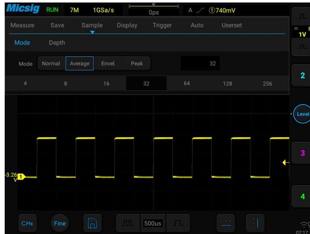
Figure 11-7 Waveform after choosing the average sampling mode, with average number 32
