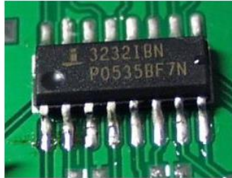
Too much solder
