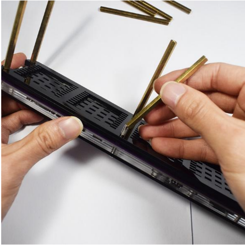
Fixed-length copper pillars;
