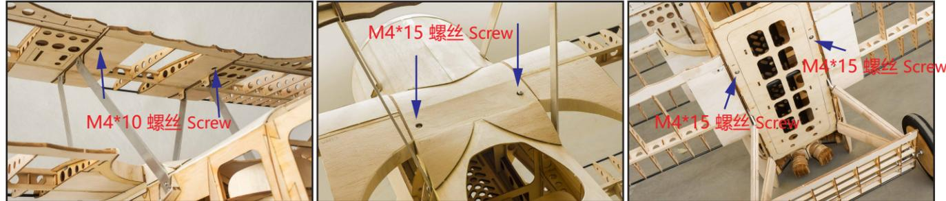
机翼支架安装图示 Wing's bracket installation show
