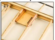
Assemble the left and right wing, connect both with the carbon tubes as picture shown below, glue at the joints.
