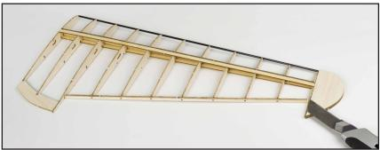
Paste the balsa cover onto the wing.
