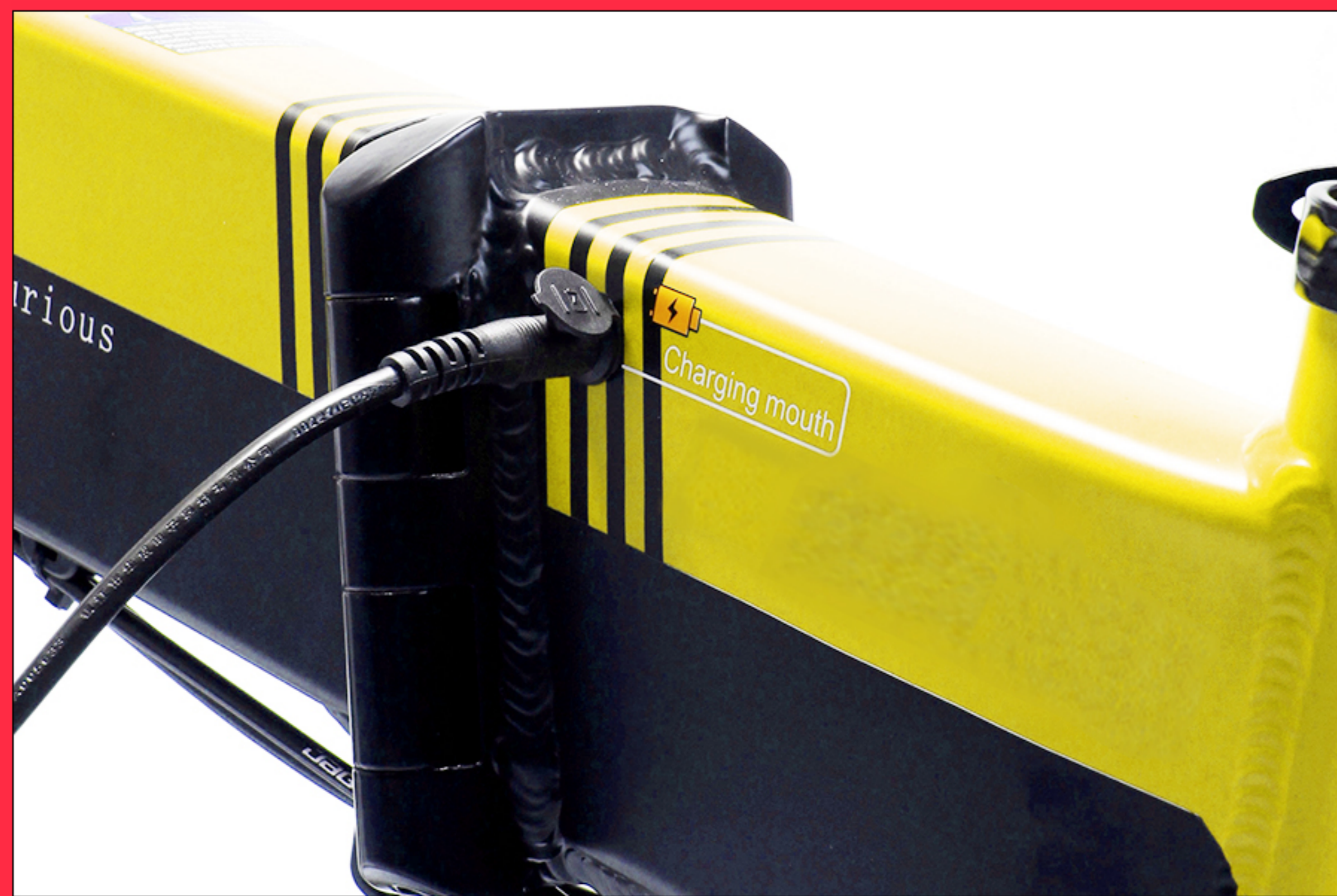
A. Recharge the battery on E-Bike directly
