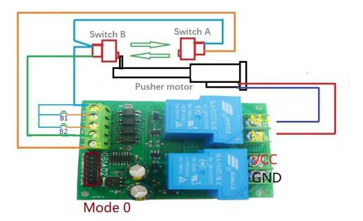
Trigger B1 to start the forward rotation push rod and extend until it touches the Switch B limit switch
