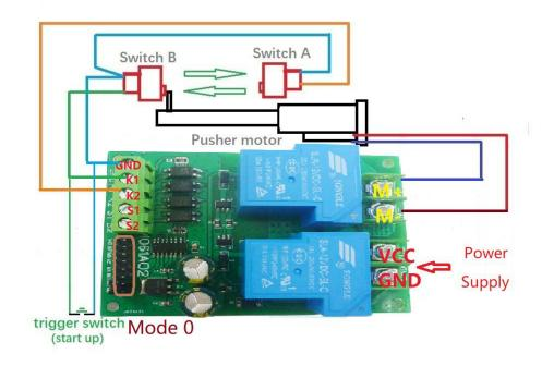
Cycle mode: no action when powered on, trigger the "trigger switch" will go back and forth between the two limit switches A and B, and cycle all the time Wiring Diagram 2: Positive and negative start independently, each time running a single pass
