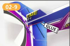
把水平尾翼插入机身尾部, 连接处用泡沫胶粘固。 Insert the horizontal tail into the tail of the fuselage, and fix the joint with foam glue.
