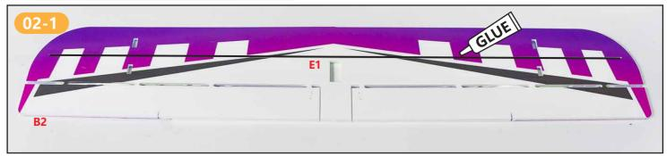
在下机翼B2底面预留槽内嵌入E1碳片,并用泡沫胶把碳片粘固在槽内。 Insert the E1 carbon sheet into the reserved groove on the bottom of the lower wing B2, and fix the carbon sheet in the groove with foam glue.
