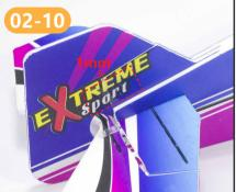
如左图,在转向舵上贴一段透明胶,然后把转向舵粘贴到机身尾翼上。保留1mm间距。 As shown in the left picture, paste a piece of transparent glue on the steering rudder, and then paste the steering rudder to the tail of the fuselage. pls take care to keep 1mm spacing.
