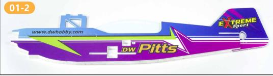
把涂好胶水的A1粘到A2的两侧,粘 贴时对齐边缘及各对应的空位。 Paste the glued A1 to both sides of A2, and align the edges and corresponding spaces when pasting.
