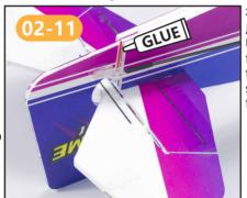
在转向舵下方与机身连接处,用少量泡沫胶粘连。 Use a small amount of foam glue at the connection point under the steering rudder and the fuselage.
