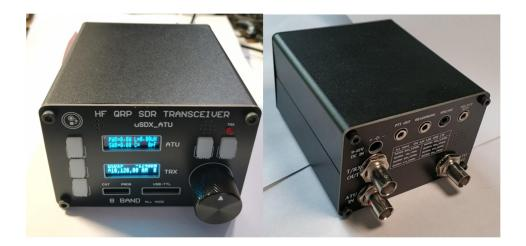
uSOTA\_+ATU is modified from uSDX SOTA ATU open source hardware designed by WB2CBA.uSDX SOTA\_ATU modifying a QCX transceiver for SDR SSB based on the open source work QCX-SSB and Automatic Antenna Tuner Unit is a miniaturized clone of David Fainitski, N7DDC's infamous 7X7 automatic antenna tuner unit adapted for QRP operation up to 10 watts.
