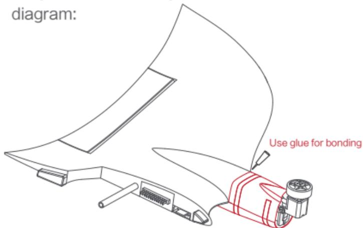
Note: Use adhesive to bond the upper and lower covers of the fairing, and use stickers to secure them tightly.
