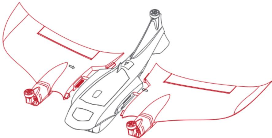
Note: Insert the wings into the fuselage on both sides to complete the assembly.
