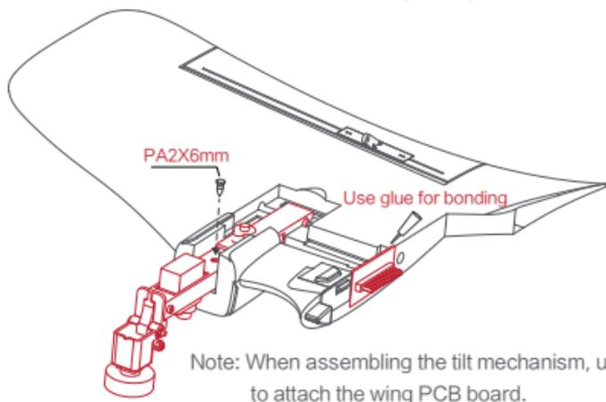
2. Installation of Wing Joining Rod is as shown in the following diagram:
