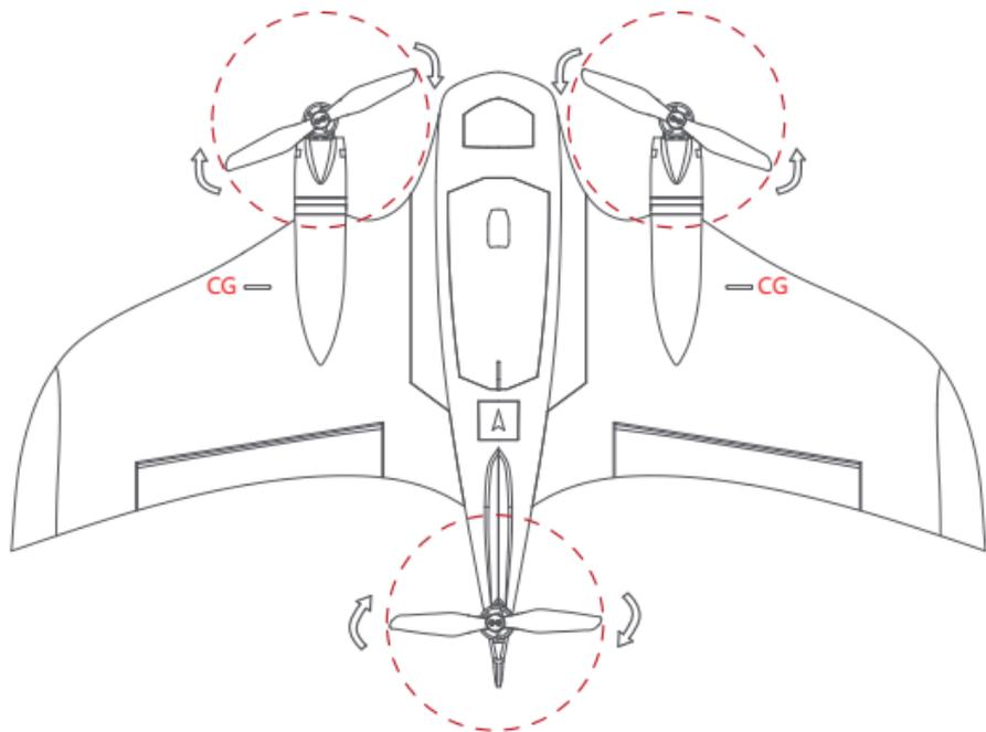
Note: As shown in the diagram, when installing the propeller blades, follow the schematic to correctly install them according to the rotation direction. Use HM2x8mm screws for installation.
