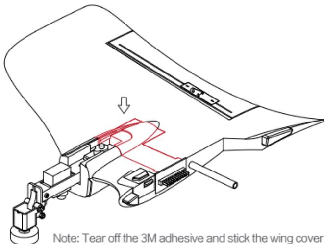
Note: Tear off the 3M adhesive and stick the wing cover in place.
