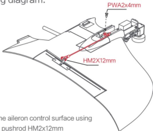
Note: Assemble the aileron control surface using the ball head pushrod HM2x12mm
