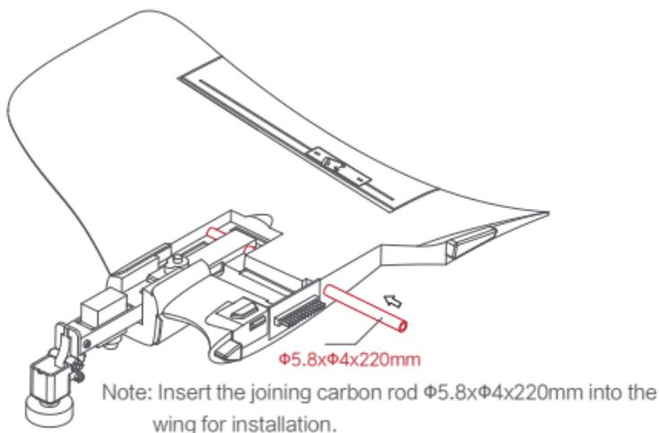
3. Installation of Wing Cover is as shown in the following diagram:
