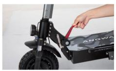
Step 2 Pull down the silver buckle, at the same time Fold or Unfold the scooter.
