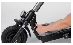
Notice: After folding or unfolding the scooter, please press the red buckle tightly into the groove to avoid loosening.
