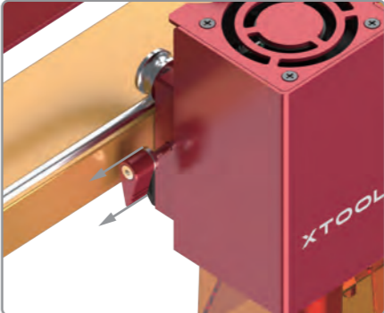
Hold the handle to draw it away from the thread part
