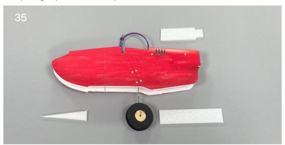
36. Use glue to secure the bottom plate of the motor compartment.
