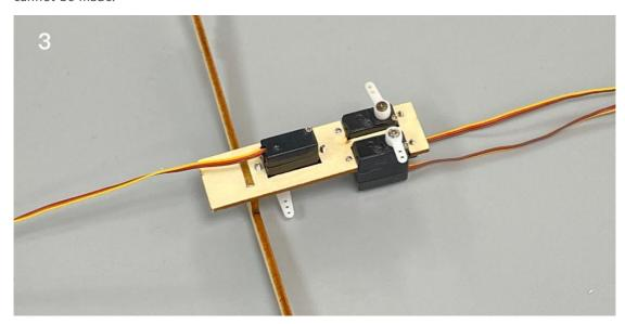
4. (Bottom view) Install and secure all three servos from underneath the wooden board.
