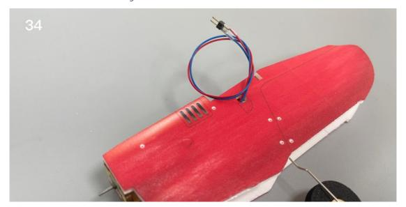
35. Press the top and bottom plates of the motor compartment and bend them into the corresponding shape of the motor compartment contour.
