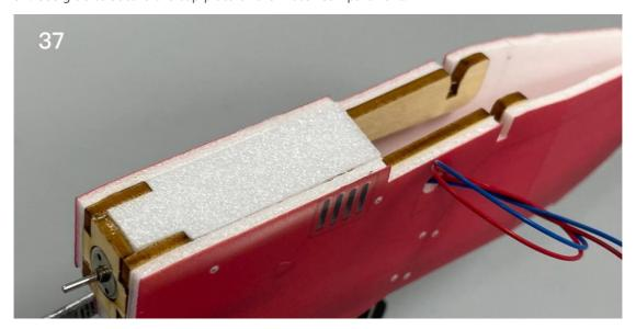
38. Install the completed motor compartments on both sides in a mirrored symmetrical manner.
