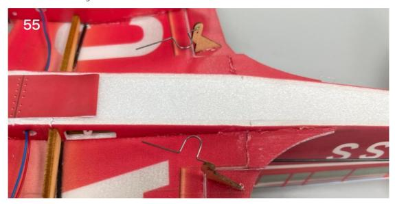
56. Insert the wire clips into the fuselage as shown in the picture and attach them onto the aileron servo arms.
