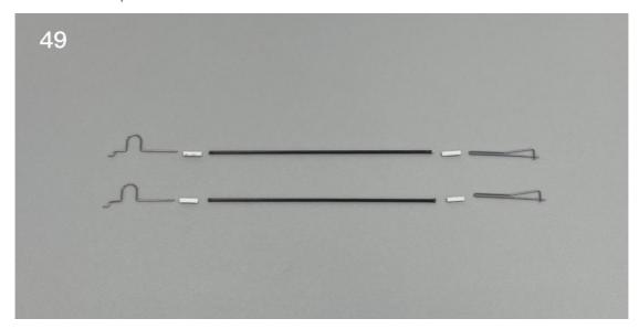
50. Use heat shrink tubing to connect the control rods to the steel wire clips and secure them with epoxy adhesive.
