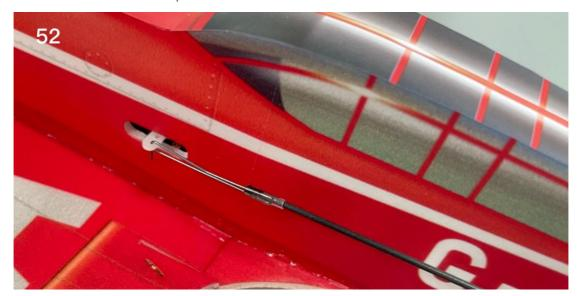
53. Trim the carbon fiber rod to an appropriate length. Use heat shrink tubing to connect the carbon fiber rod to the connecting hook and secure it with epoxy adhesive.
