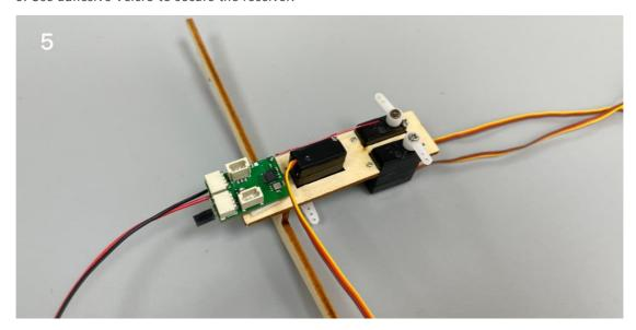
6. Connect the receiver to the servos. Turn on the transmitter and test the correspondence between the three servos and the channels on the transmitter.
