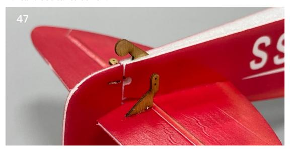
48. Install the rudder control horn.
