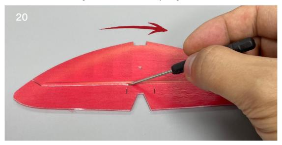
21. Use a sharp tool (screwdriver) to score through the marked lines on the bottom of the vertical stabilizer, allowing the rudder to move freely along the lines on both sides.
