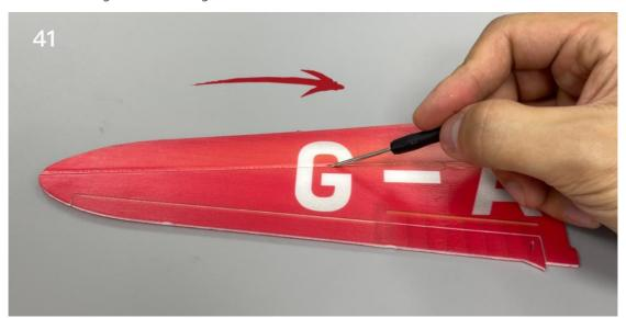
42. Use a sharp tool (screwdriver) to score along the aileron's marked line, allowing the aileron to move up and down along the line.
