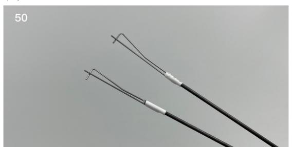
51. Install connecting hooks on the tail control horns.
