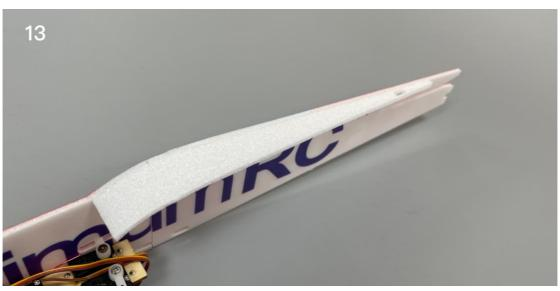
14. Use glue to secure the front top plate of the fuselage.
