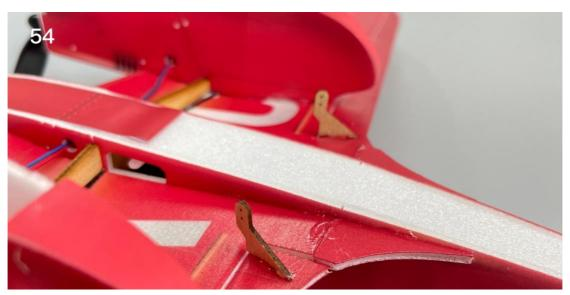
55. Install connecting hooks on the aileron control horns.
