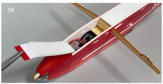
20. Use a sharp tool (screwdriver) to score through the marked lines on the bottom of the horizontal stabilizer, allowing the elevator to move freely along the lines on both sides.
