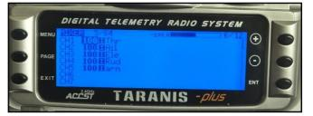
3. The default channel map for Mobula6 Frsky version is TAER 1234, please make sure your transmitter is matched, otherwise it will can't be armed. Toggle the AUX1 Switch, the Green LED on the flight controller will getting to be solid, this indicates the motor was armed. And also you can found "Armed" displayed on your FPV Goggles or the FPV Monitor. Please make sure keep the Mobula6 level before arming .Be careful and enjoy your flight now !
