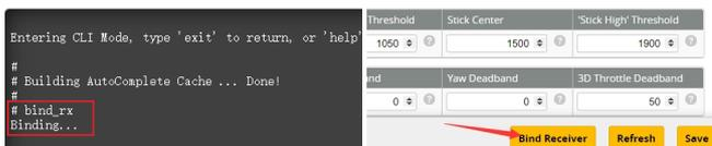
3.Make your Flysky transmitter to bind mode, the LED at the bottom of the flight controller will getting to be solid if bind successfully. The Default SPI receiver protocol is AFHDS2A, so please check your radio transmitter is matched.
